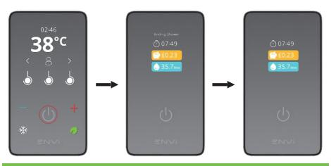
ENVi® can calculate and display the cost of showering at the end of every session! This can be enabled by entering Energy and Water Unit Prices in the System Settings (pg.14).
