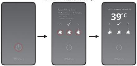
Touch the circular symbols under the  $\wedge$  and  $\vee$  chevrons to navigate menu items, and use the circular symbol under the  $\checkmark$  to confirm selection.
