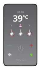
Touch the circular symbols under  $\langle$  and  $\rangle$  chevrons to select a User Profile and touch the circular symbols under  $\checkmark$  to confirm
