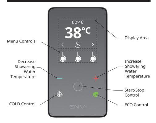
The function of each **Menu Control** adapts to the mode it is used in, and is denoted on-screen above each control by one of the following icons:
