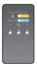
The cost of showering is calculated using the total water and energy used per shower, along with the unit prices for each. Any adjustment to the Energy or Water Unit Price is not retrospective and only applies when calculating the usage of future showering sessions.
