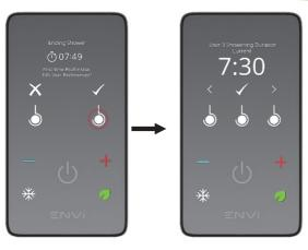
When ending a shower with a User Profile selected for the first time, the shower displays an option to navigate to the User Profile Settings menu for that User Profile, so that it can be personalised. Touch the circular symbols under the ✓ to navigate to the menu, or touch the circular symbol under the ✗ to advance to the shut down screen.
