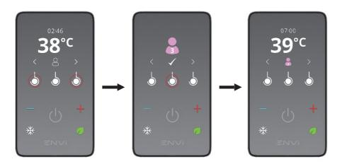
Upon selecting a User Profile, the shower will automatically adjust the shower temperature and reset the timer to the personalised settings for that User Profile. The shower temperature can still be manually adjusted by touching the — and — controls.
