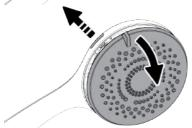
Release the button and gently pull the face plate away from the body using the adjustment lever.
